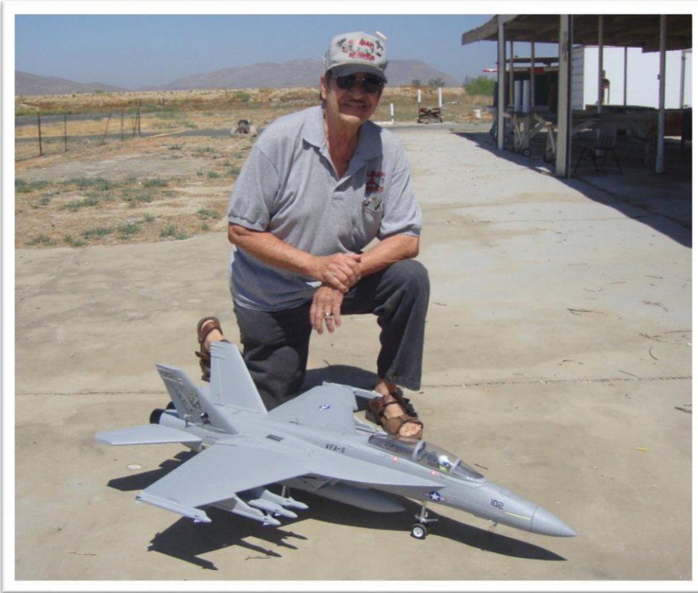
Bob Estrella with his FMS F/A-18F EDF. It's powered by a 6 Cell 3300mah Lipo.
